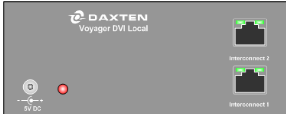
Front & Rear Panel Layout Voyager DVI Dual head USB – Local Unit
