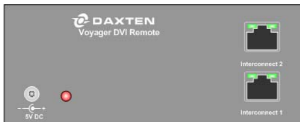
Front & Rear Panel Layout Voyager DVI Dual head PS/2 – Remote Unit
