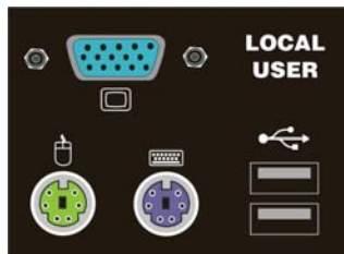
Figure 51 Local User Panel on Dominion KX
